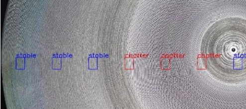
Figure 5.4: Product turning surface after roughness measurement and marking of stable and vibrating regions
