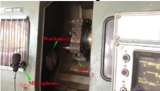
Figure 3.7: sound collection during flange facing turning process
