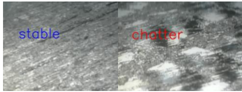
Figure 5.7: Vibration recognition during turning process
