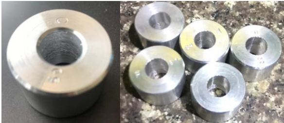
Figure 6.9: Vibrating machined products with magnetic field effect
